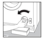
Unscrew and remove the filter.
